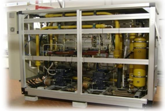
CO2 Refrigeration System Test Rig
